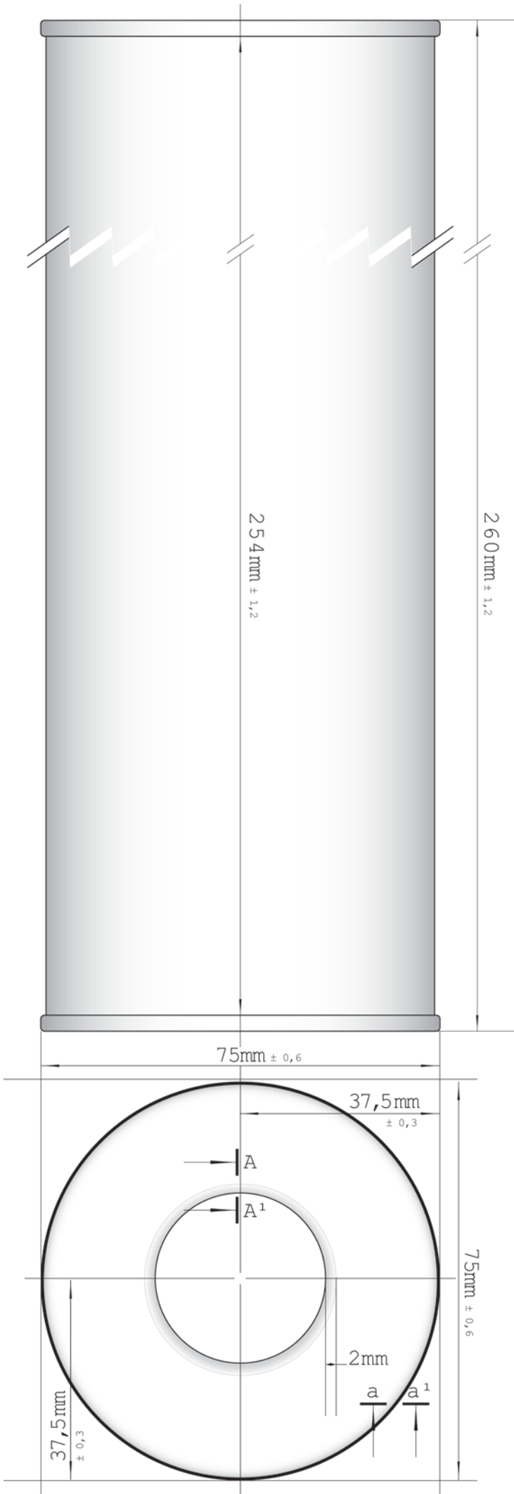
3-PIECE TIN CAN 1000ml TECHNICAL DRAWING DIA. Ø73mm
